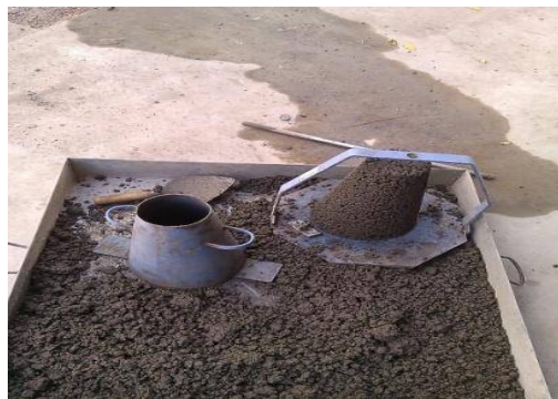
Fig 2.1: slump cone test
