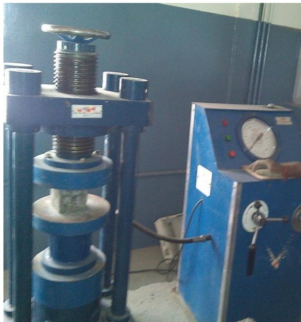
Fig 2.3: testing of the cube in compressive machine
