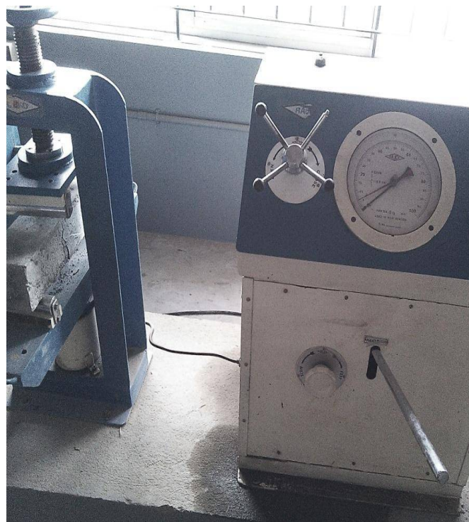
Fig 2.4: testing of concrete beam in flexural testing machine
