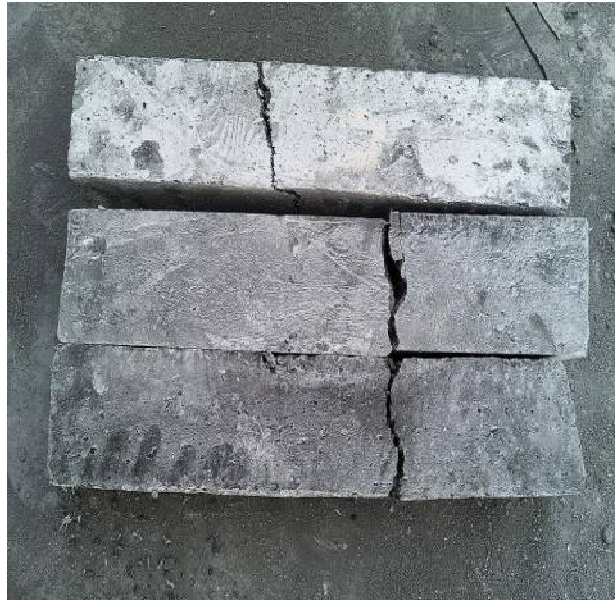
Fig 2.5: Concrete beam after testing in flexural testing machine
