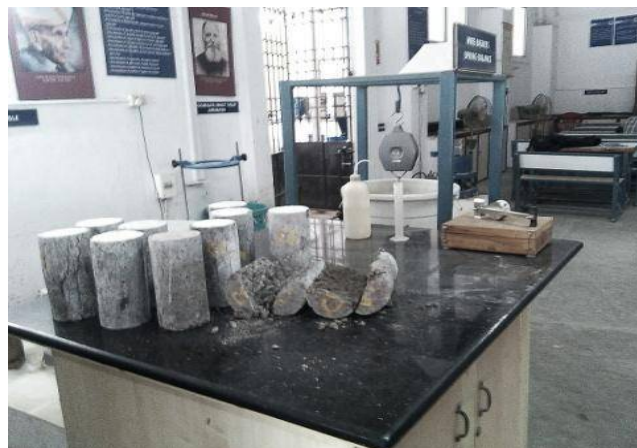
Fig 2.6: Cylindrical specimen after split tensile strength test.
